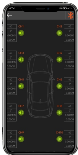
Chanel: Press Channels ico You will see the interface, you can set each channel's Gain/Phase/Time delay/Open/close volume.
